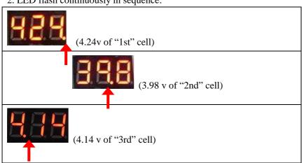
\* When the is less than 3cell connected, i.e. test a 2S pack:
